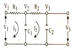
2. Develop a model for the physical system shown below using bond graph
