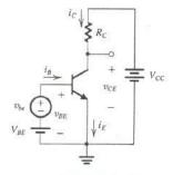
a. 5. For the circuit shown in the figure select a value for RB so that the transistor saturates with an overdrive factor of 10. The BJT is specified to have a minimum  $\beta$  of 30 and VCEsat = 0.2 V. What is the value of forced  $\beta$  achieved?
