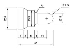
2. Write a cnc code for the following profile with an aluminium work piece. Calculate the spindle speed. cutting velocity of aluminium is 80 MPM.
