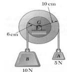
4. For the drum and flywheel, I=10.5 kg-m2. The bearing friction is equivalent to a couple of 60Nm .At the instant shown, the block is moving downward at 6 m /s. Determine the velocity of the block after it has moved 4 m downward.
