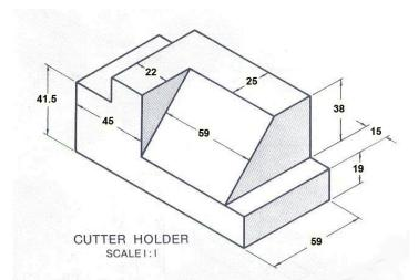
2. Draw the orthographic views for the given 3D model with appropriate dimensioning using CAD package.
