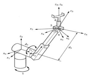
3. Determine the kinematic parameters for the PUMA 260 robot and derive the complete forward kinematics equations for the center of the wrist by establishing the DH frames, finding and taking the product of the corresponding homogenous transformations
