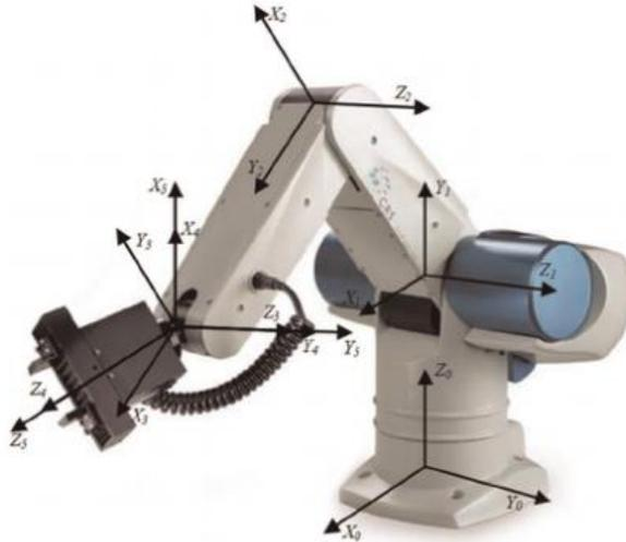
2. Find the DH parameters for the robot given in the following fig and derive the forward kinematics
