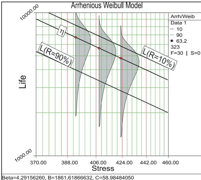
**Figure 13: The Arrhenius relationship linearized on log-reciprocal paper.**
