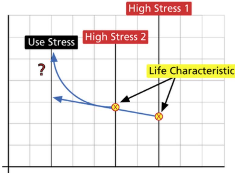
The life characteristic can be any life measure such as the mean, median,  $R(x)$ ,  $F(x)$ , etc. This life characteristic is expressed as a function of stress. Depending on the assumed underlying life distribution, different life characteristics are considered. Typical life characteristics for some distributions are shown in the next table.
