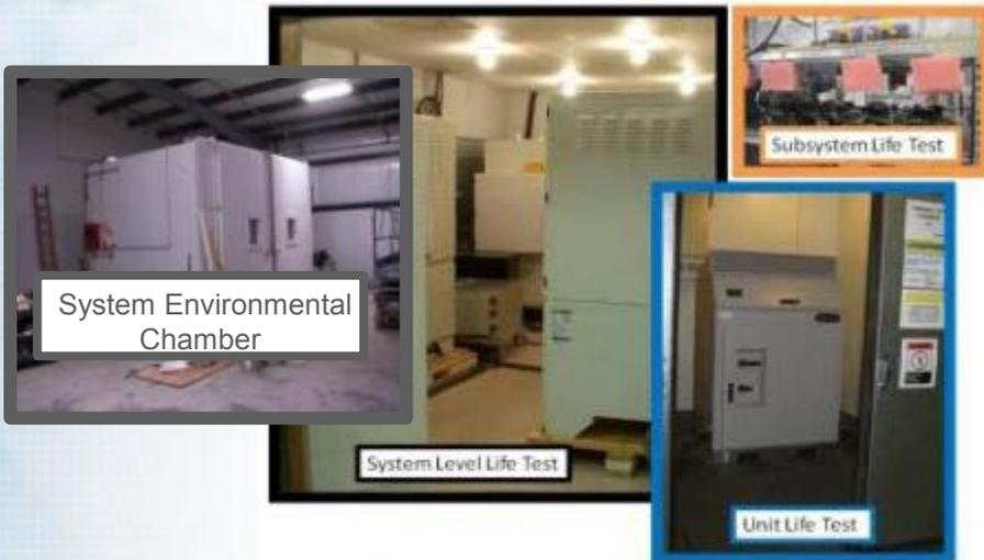
AE has performed ALT for up to two calendar years upon inverters at 50degC, 24X7
