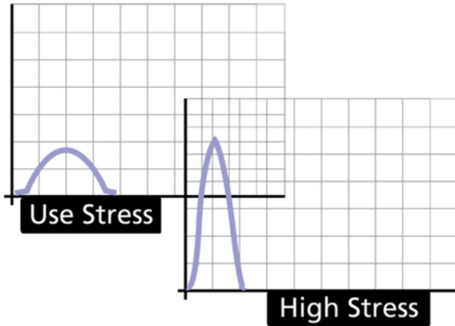
To further simplify the scenario, let's assume that the *pdf* for the product at any stress level can be described by a single point. The next figure illustrates such a simplification where we need to determine a way to project (or map) this single point from the high stress to the use stress.
