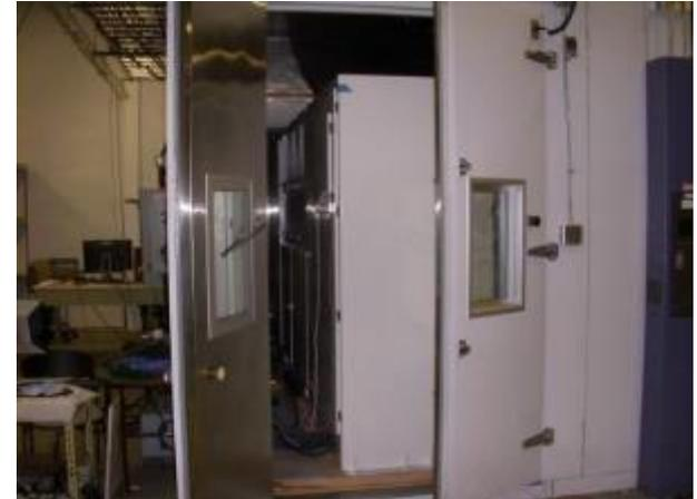
Anderson Electric Controls Supply and Solar Simulator Inverter housed within AE environmental chamber
