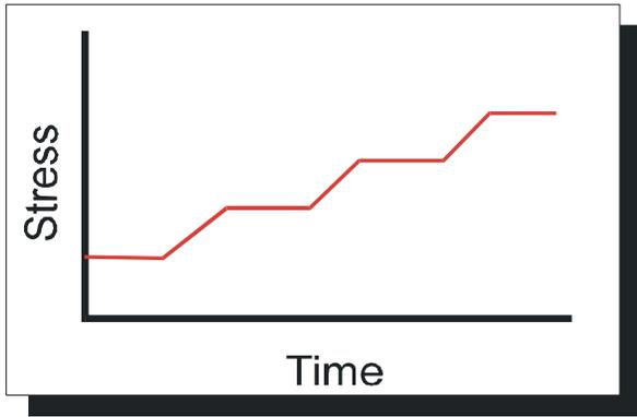
Figure 10: Graphical representation of the ramp-stress model.
