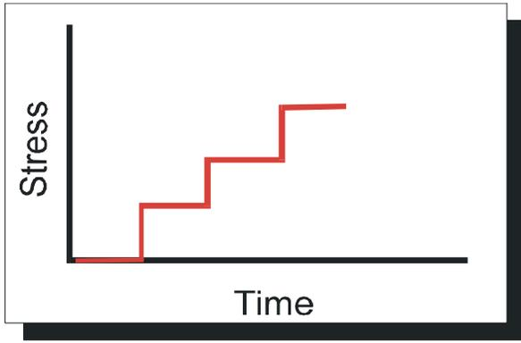
Figure 9: Graphical representation of the step-stress model.
