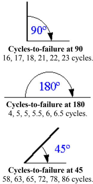
The accelerated test data were then analyzed in [10], assuming a lognormal life distribution (fatigue) and an inverse power law relationship (non-thermal) for the stress-life model. The analysis and some of the results are shown in the next figures. The base data were analyzed using [12] and a base MTF estimated. In this case our accelerated test correctly predicted the MTF as verified by our base test.
