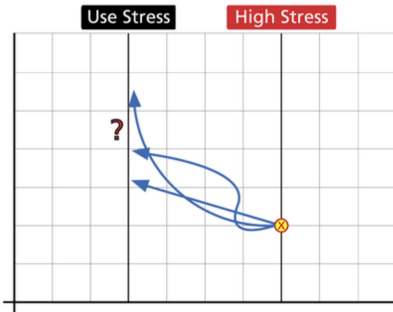
Obviously, there are infinite ways to map a particular point from the high stress level to the use stress level. We will assume that there is some model (or a function) that maps our point from the high stress level to the use stress level. This model or function can be described
