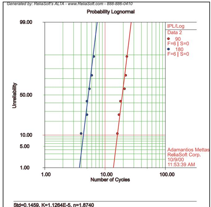
Figure 22: Resulting Probability plot for 90 and 180 bends.
