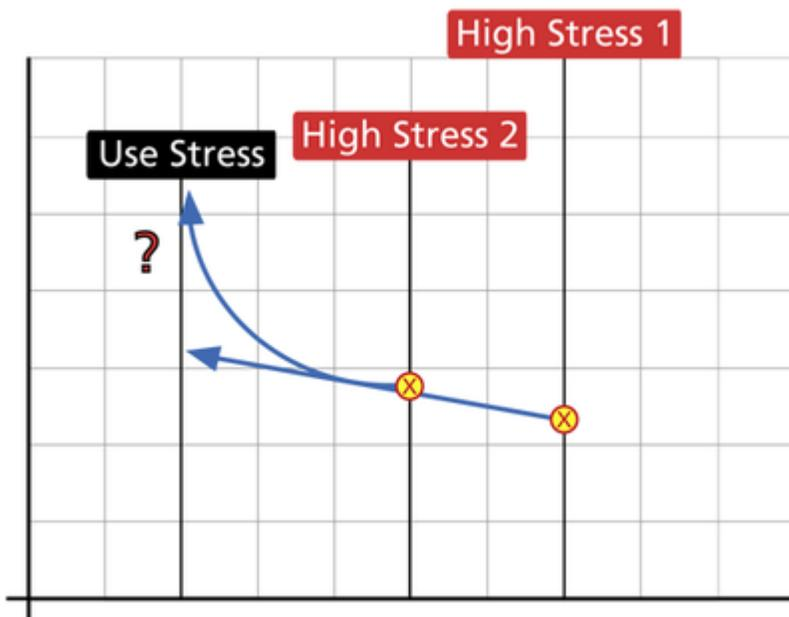
The above figure illustrates that you need a minimum of two higher stress levels to properly map the function to a use stress level.
