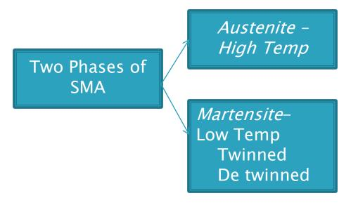
A phase transformation which occurs between these two phases upon heating/cooling is the basis for the unique properties of the SMAs.
