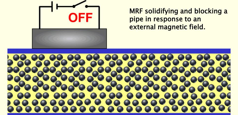
"OFF" position – the MR fluid is not magnetized & the particles inside, distributed randomly, allow the fluid to move freely, acting like a damper fluid.
