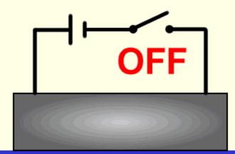
MRF solidifying and blocking a pipe in response to an external magnetic field.
