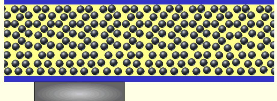
**"OFF" position** – the MR fluid is not magnetized & the particles inside, distributed randomly, allow the fluid to move freely, acting like a damper fluid.
