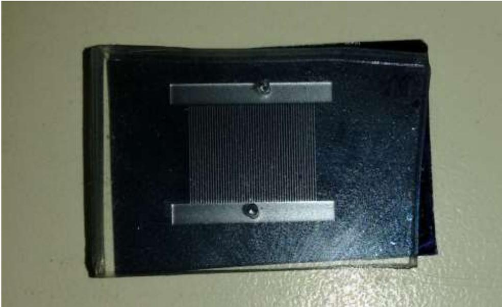
Fig. 5.9. PDMS layer bonded with Silicon substrate
