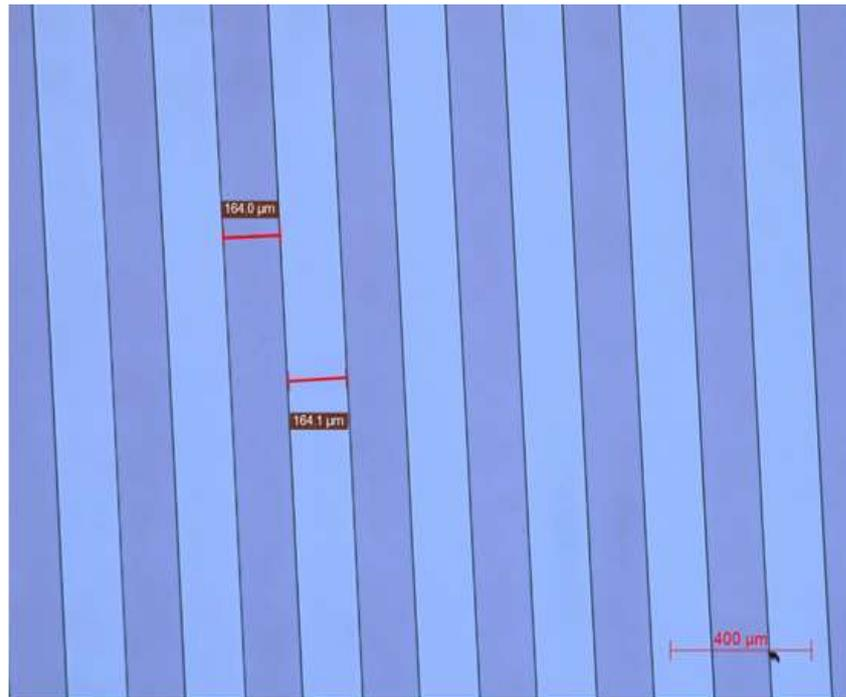
Fig. 5.5. 150 μm Channel view after RIE
